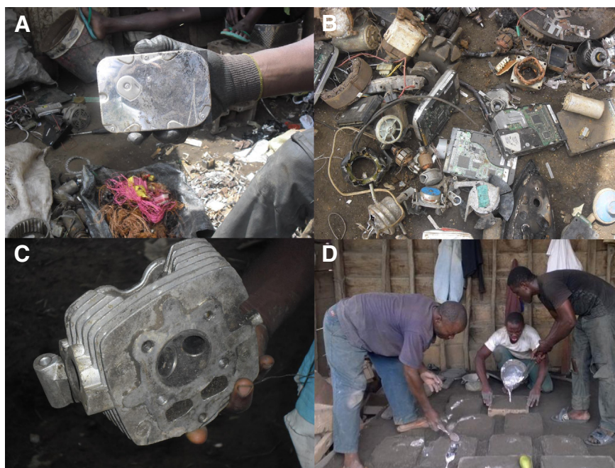
Fig. 1. Some source materials used in the manufacture of artisanal aluminum cookware in Cameroon. (A) Computer hard drive cover; (B) mixed scrap including computer parts; (C) motor bike engine part; and (D) molten scrap being poured into molds for pots.
