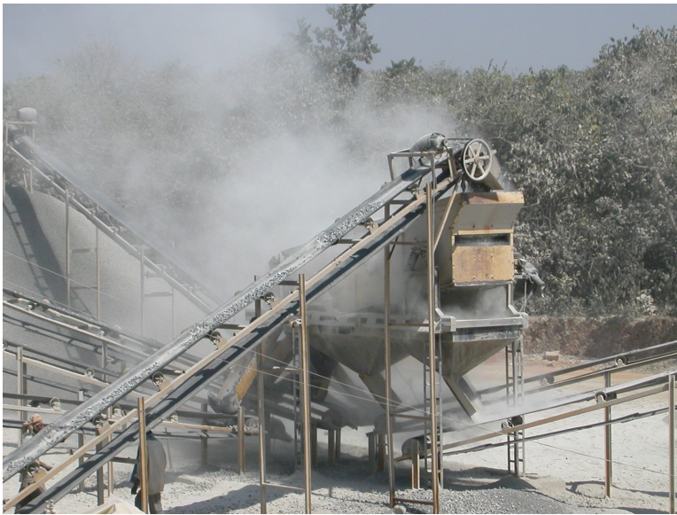
Figure 1. Stone crushing operations create large quantities of respirable dust. Workers exposed to respirable silica dust have an increased risk of developing lung diseases such as silicosis or tuberculosis.
