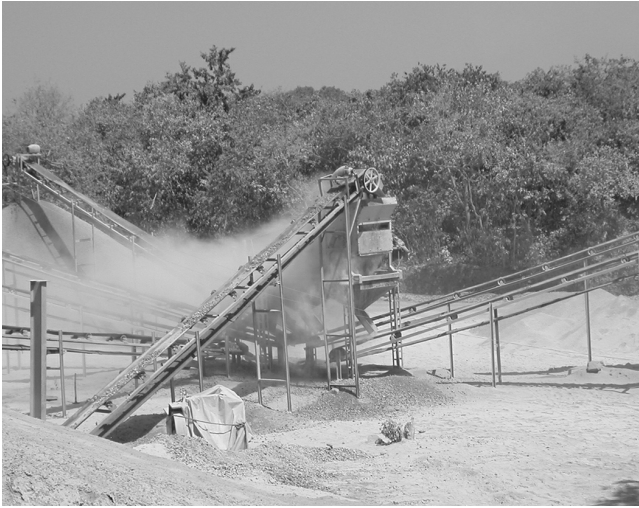
Typical stone crushing operation without containment. Large dust plumes are created during the crushing process.
