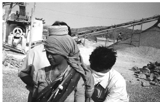
Worker being fitted with air sampling pump for sampling respirable silica concentrations.
