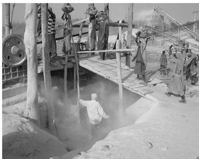
Stone crushing units are labor intensive. These units are often located in tight clusters and dust drifts from neighboring operations.
