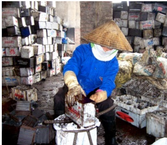
Lead Batteries being Dismantled for Recycling in Vietnam
