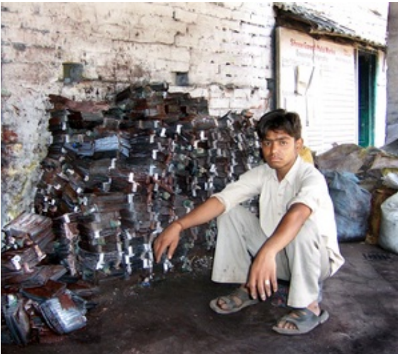
Lead Plates from Used Batteries in one of Kolkata, India's Recycling Plants
