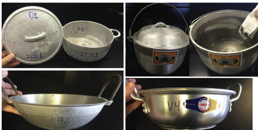
Fig. 1. Photos of representative cookware items (clockwise from upper left) from (a) Ivory Coast; (b) Philippines (with inset showing pot after boiling with dilute acetic acid); (c) Viet Nam; and (d) Bangladesh. (For interpretation of the references to colour in this figure legend, the reader is referred to the web version of this article.)
