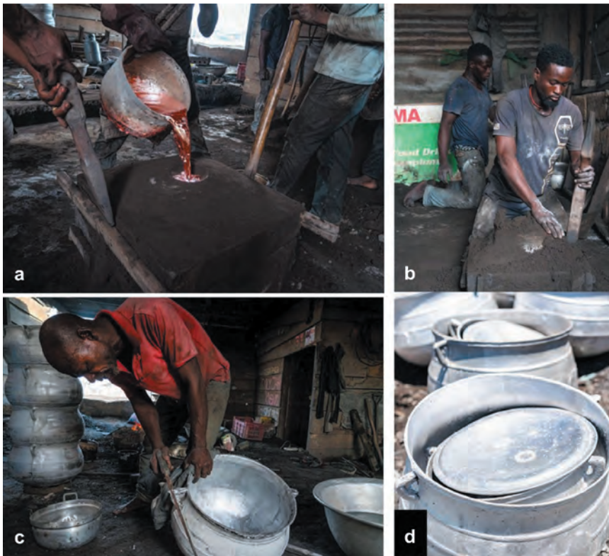
Figure 3. (a) Melted metal being poured into sand mold to produce pots. the coppery appearance of the molten metal is from an engine block. (b) Artisan is creating a sand mold. (c) Rough edges and other defects are removed before finishing the pots. (d) Finished pots for sale in local marketplaces.
