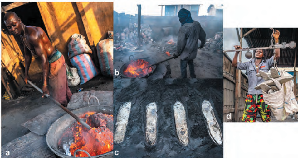
Figure 2. Photos of aluminum recycling and artisanal cookware production. (a) Air conditioner fins being melted down. (b) Melting of plastic-coated blister foils produces noxious fumes. (c) Scrap is initially melted into ingots which are (d) sold by weight to cookware artisans.
